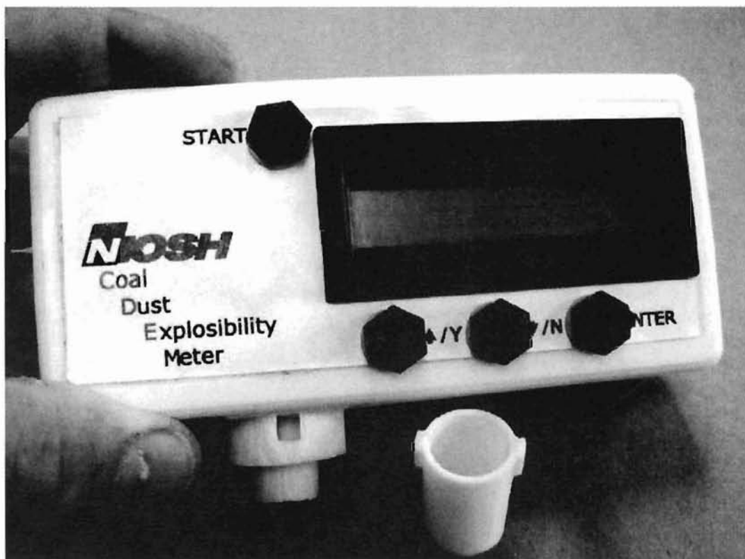
Figure 4. Coal Dust Explosibility Meter (CDEM).
