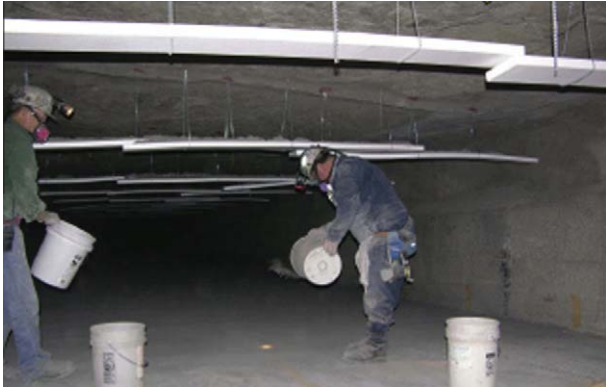
Fig. 5. Example of coal and rock dust being suspended from the mine roof and placed on the mine floor.
