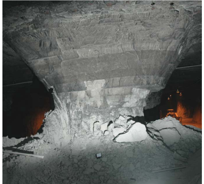
Fig. 4. Pillar that had an original width-to-height ratio of 1.7 failed by progressive spalling. Thin weak beds are thought to have contributed to the failure. Average pillar stress is about 11% of the UCS.
