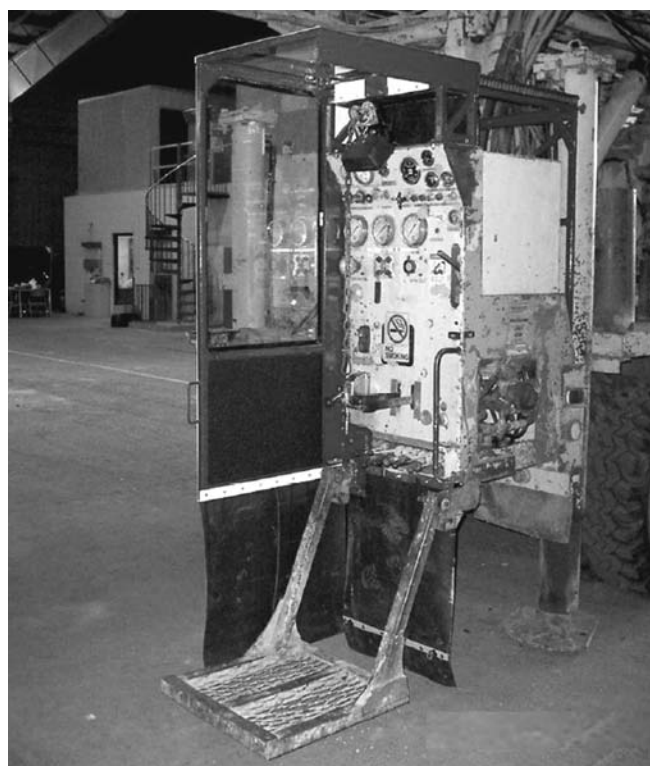
Figure 15 — Completed partial cab installed on the drill rig.
