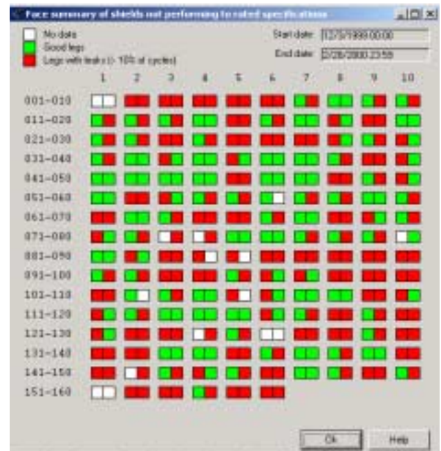
Figure 9. A grid can be displayed which also provides an overall summary of the complete face. In this case, shields with and without leaking cylinders are identified.
