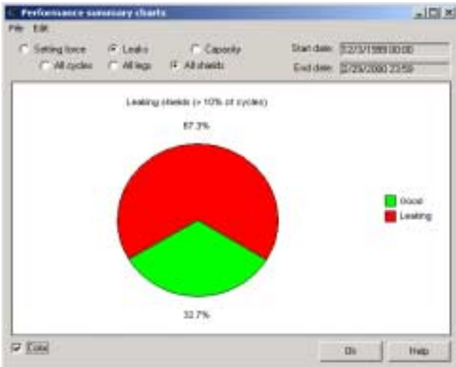
Figure 12b. As seen in this pie chart, 67.3 pct of the shields had one or more leaking cylinders.
