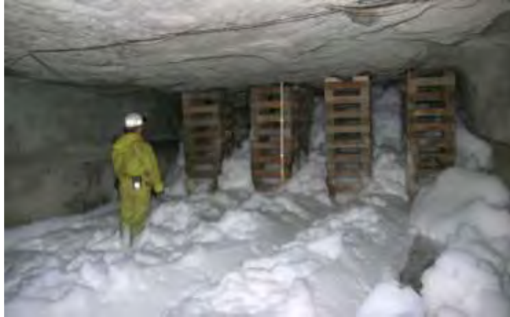
Figure 4: Compressed air gas-enhanced foam accumulating behind and moving through crib block sets at the LLEM (Smith et al. , 2005).
