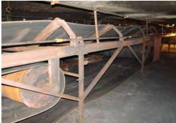
Figure 3: Conveyor belt fire suppression system set-up at the NIOSH Fire Suppression Facility (Rowland III et al , 2009).
