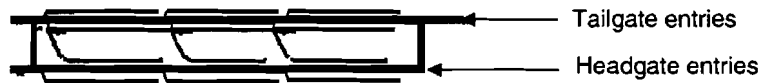
Fig. 11. An example layout showing additional horizontal, in-seam boreholes on either side of the gateroads in addition to pattern A. The entries represent a three-entry system with intervening coal pillars.
