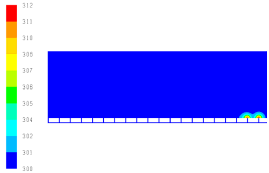
Figure 12 Temperature distribution (K) in the gob after 15 days with the leakage rate of 0.047 \text{ m}^3/\text{s} at two seals.
