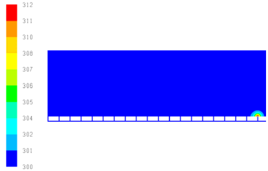
Figure 11 Temperature distribution (K) in the gob after 15 days with the leakage rate of 0.047 \text{ m}^3/\text{s} at one seal.
