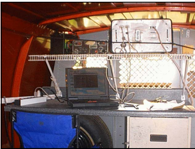
Figure 9.—Data acquisition system with electrode scanner (upper right), ABEM 300-C geoelectrical resistivity instrument (upper middle), auto battery (upper left), and laptop computer (lower middle).
