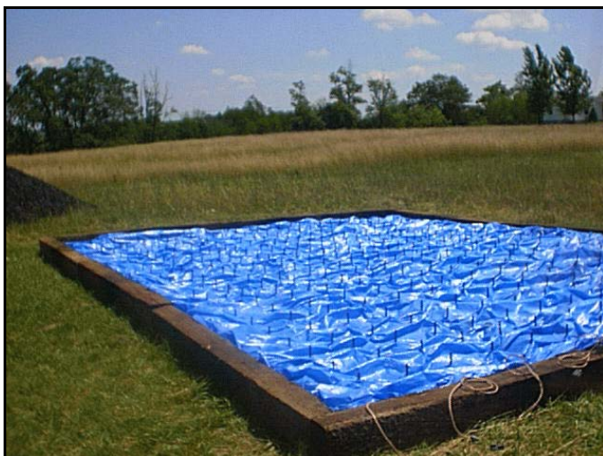
Figure 5.—Completed grid showing insulator plastic tarp ground cover, frame reinforced with railroad ties, and some of 15 electric cable lines
