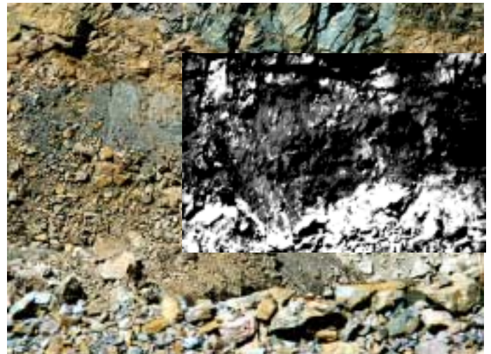
Figure 4. Results from the CMRI spectro-polarimetric imager. Light areas correspond to ore; darker areas to waste or unclassified spectra.
