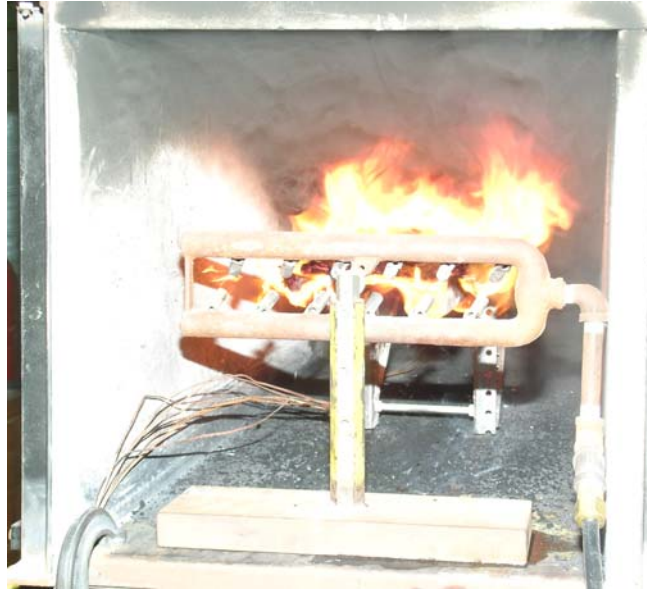
Figure 2. The ventilated tunnel with the gas burner igniting a sample belt
