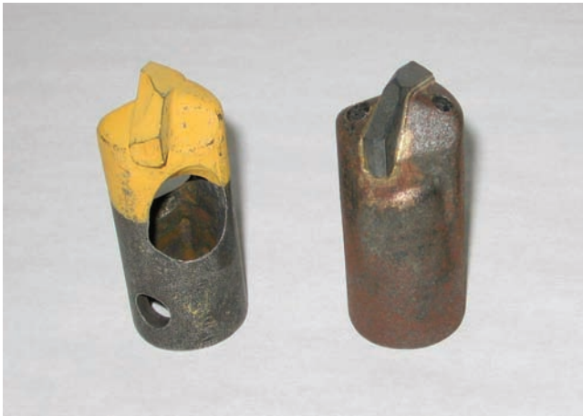
Vacuum drilling bit (left) and mist drilling bit (right).
