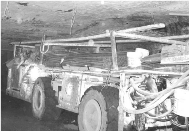
Fig. 7. Roof bolter with rails for storage of roof screen (Compton et al., 2007).
