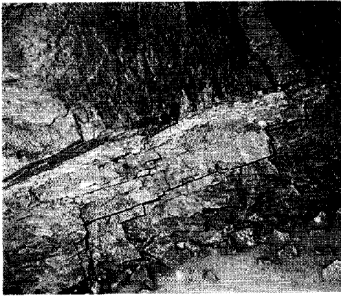
Figure 2. Soft, white gouge on slip plane in argillite interbedded in hanging wall rib.
