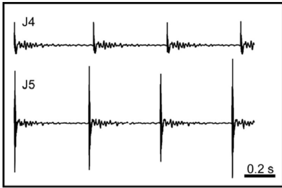
Figure 5—LDV vibration signals from hammer impacts on competent (S) and damaged (L) targets J4 and J5.
