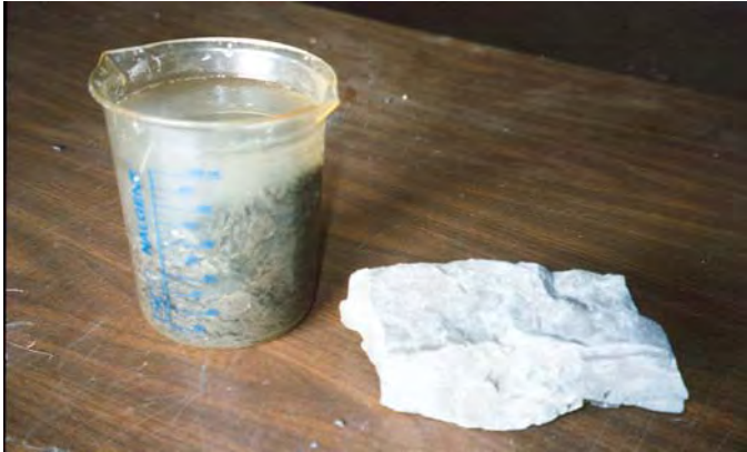
Figure 1. Immersion test showing specimen deterioration and original sample.
