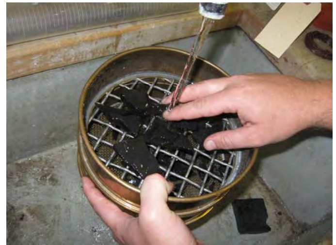
Figure 3. Wet sieving of the sample during the Consol Energy Water Sensitivity test procedure.
