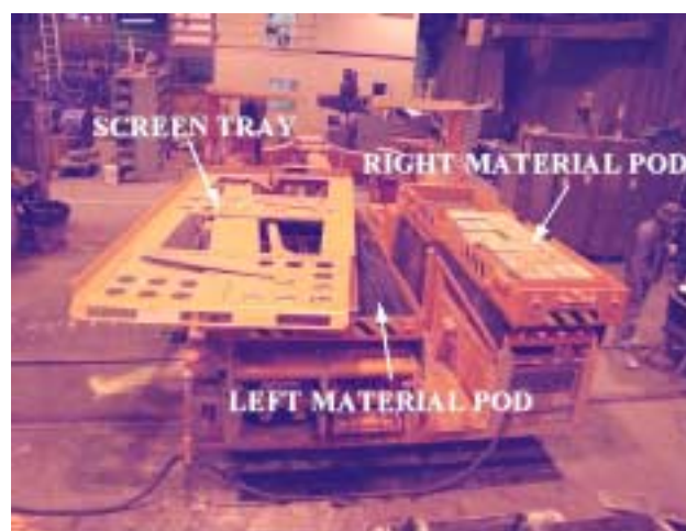
Figure 8. The J.H. Fletcher material handling system, featuring left and right material pods and roof screen tray.
