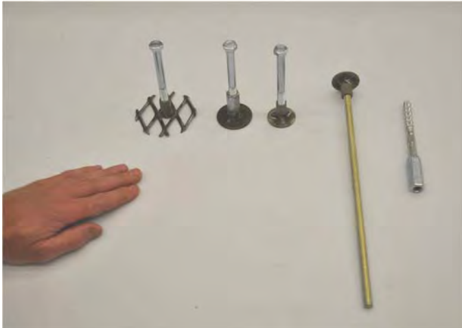
Figure 9. Pull anchors investigated during the development of a direct tensile test system for determining shotcrete adhesion strength.
