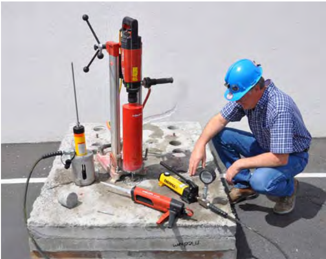
Figure 12. Field expedient direct tensile test system.
