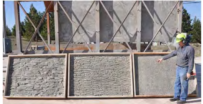
Figure 7. Concrete panels cast with three distinct surface roughness profiles.
