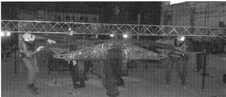
FIGURE 43.2 Test subjects remove wire mesh from actual equipment under replicated mine seam height conditions.
