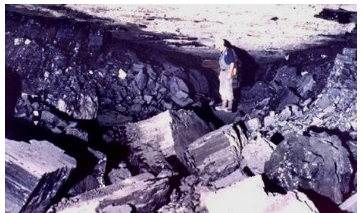
Figure 7. A coal burst has filled the mine entry with broken coal.
