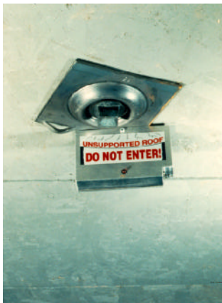
Figure 2.—Disposable magnetic-mount roof hazard alert module (9-V).
