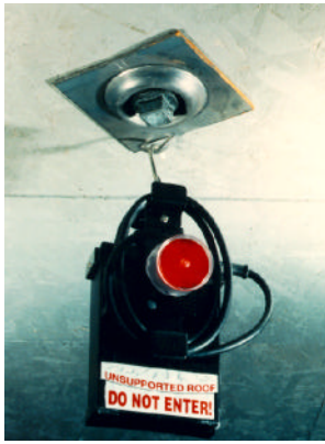
Figure 1.—Rechargeable roof hazard alert module (4-V).
