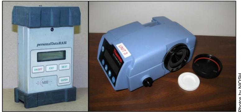
**Figure 1. Thermo Scientific's pDR-1000 sampler (left) and pDR-1500 sampler (right).**
