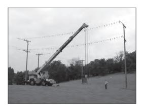
Figure 8. Full scale power line proximity alarm test at Pittsburgh Research Laboratory
