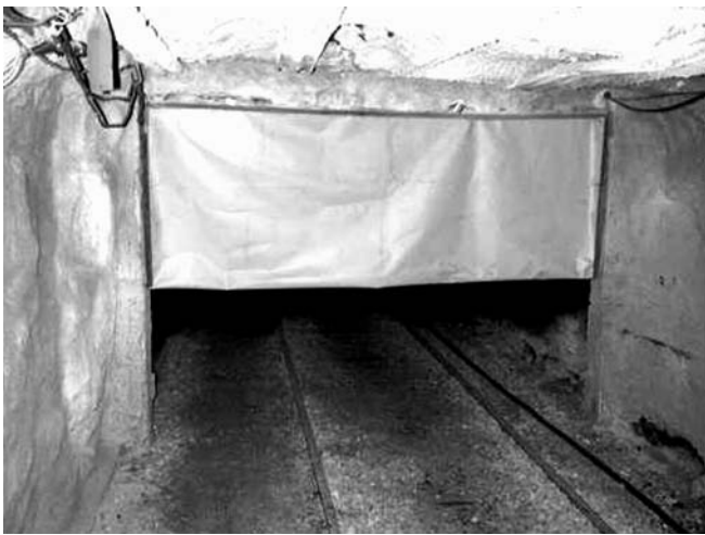
Figure 6 — Brattice blockage of smoke 29 m (95 ft) upwind from the fire in B-Butt in Experiment No. 4.
