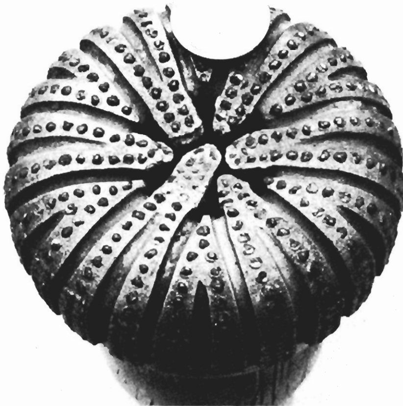
FIGURE 9. - Diamond bit. Type 147496, 76-mm (3-in) diameter.
