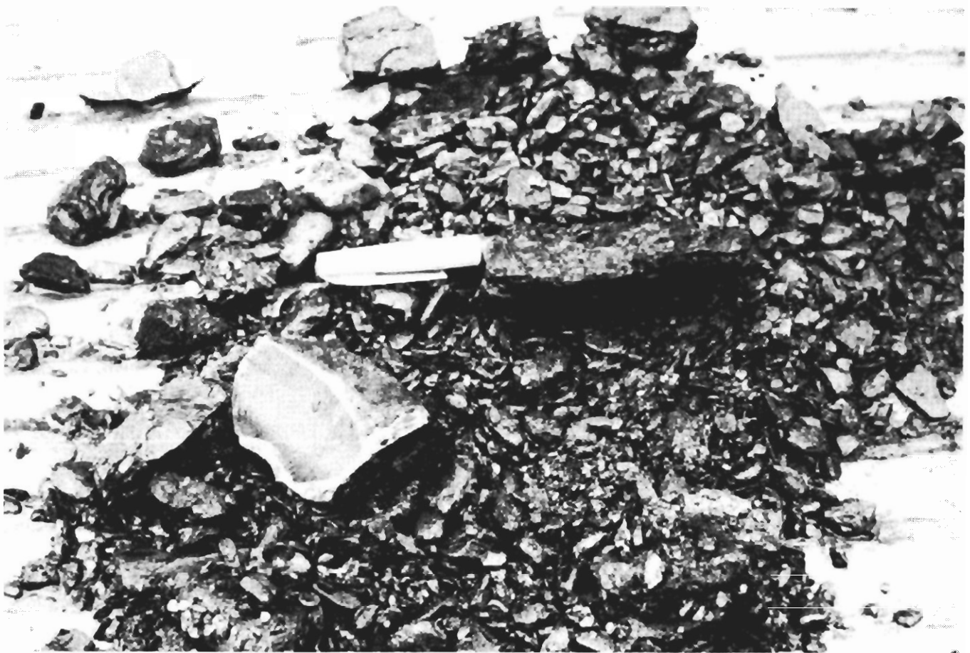
FIGURE 25. - Shale and coal blown out of EM-19, January 1980. Pen cap 57 mm (2.25 in) long. Note large cement piece.
