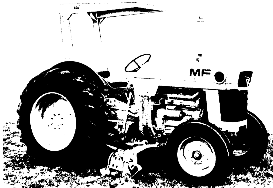
Figure 4-21. Sims Cabs, Inc. ROPS on Massey Ferguson Industrial Tractor
