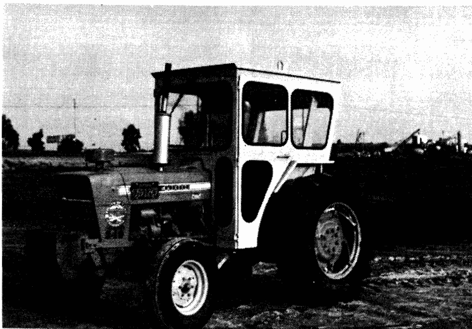
Figure 4-25. Saf-T-Cab ROPS on Euclid Off-Road Dump Trucks; ROPS Cab on Ford Industrial Tractor
