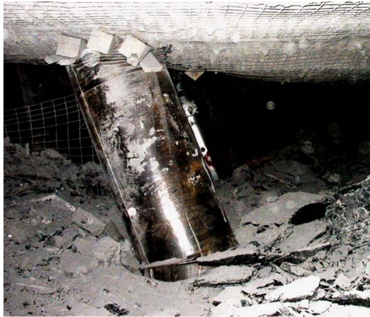
Figure 2b. The Can is the most stable support presently available. It can accommodate large roof-to-floor convergence as well as large lateral displacements.
