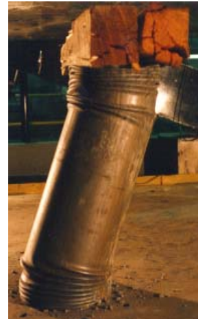
Figure 19. Biaxial loading with a ratio of 3 to 1 vertical to horizontal displacement of the support.
