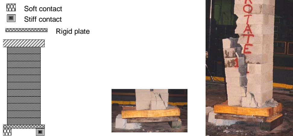
Figure 18. Floor heave simulation and examples of support testing.
