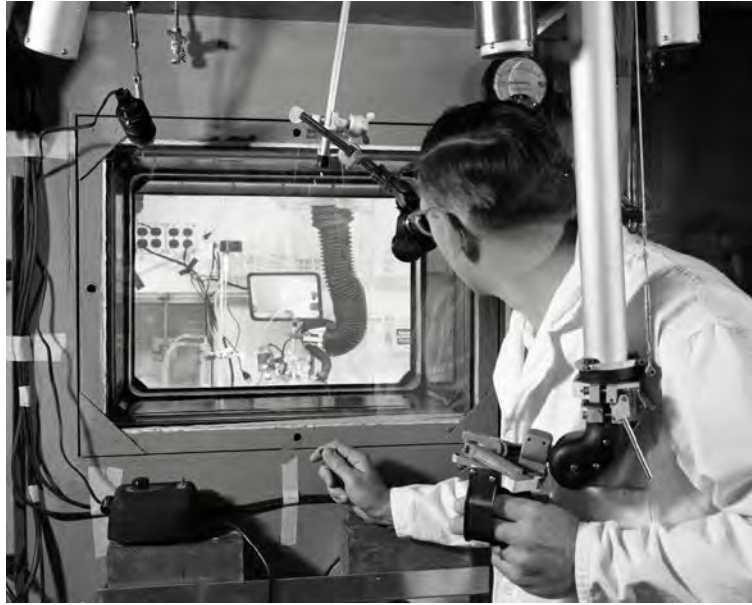
Figure 5-21: Preparation of Pure Pa-233, Alpha Cave
