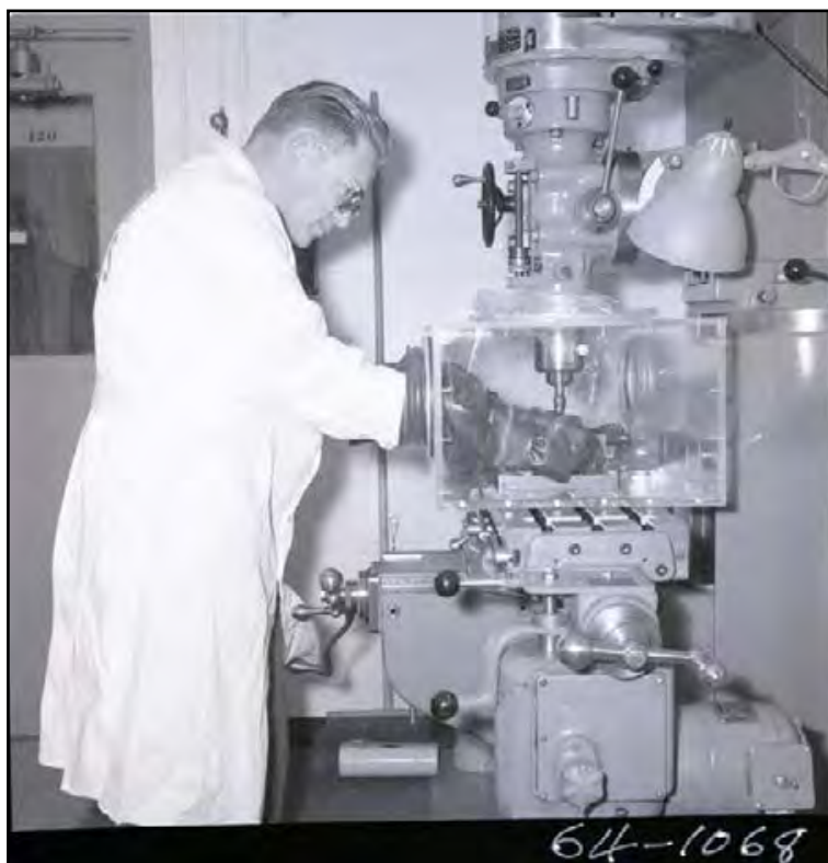
Figure 5-20: Scientist Machining Thorium, Alpha Lab, 1964
