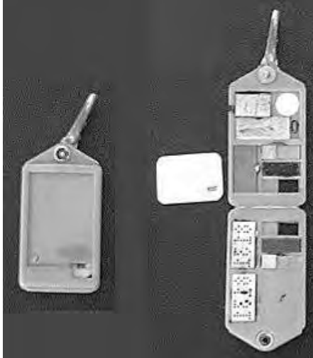
Figure 6-2. RFP multielement film badge.
