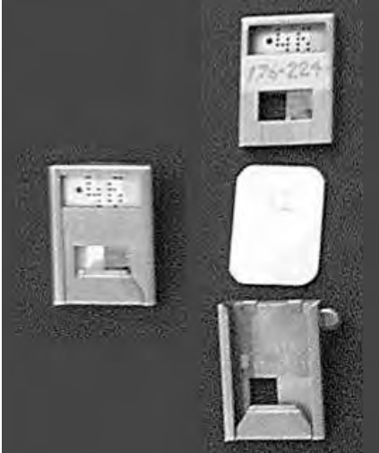
Figure 6-1. ORNL-style film badge (including brass filter).
