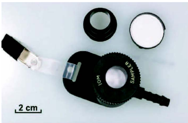
Figure 2B. IOM inhalable sampler. This is the first sampler designed specifically to match the inhalable sampling convention. The sampling cartridge is shown on the right with the inlet, filter, and support grid. All dust entering the cartridge is collected and analyzed. Sampler is made of conductive plastic and operates at 2 L/min.
