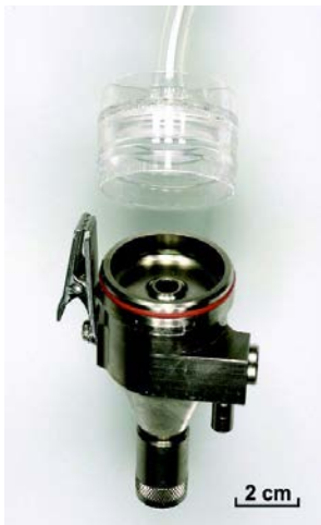
Figure 2I. GK2.69 cyclone. This cyclone was designed to match the slope of the thoracic and respirable conventions more closely than other sampling cyclones. Cyclone construction is stainless steel and operates at 4.2 L/min as a respirable sampler and 1.6 L/min as a thoracic sampler. GK4.162 RASCAL Cyclone is also available for higher flow rates of 8.5-9 L/min.
