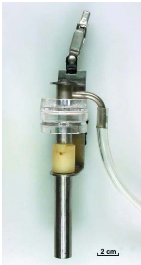
Figure 2G. Dorr-Oliver 10-mm nylon cyclone. It is used as a respirable sampler most often at 1.7 L/min. A version of this sampler is used at 2 L/min in coal mines with a 1.38 correction factor applied to the resultant mass. The holder encases body of the cyclone so that only the inlet section is visible just below the connection to the 37 mm cassette. The coal mine dust sampler version uses a cassette with an aluminum cartridge encasing the collection filter.
