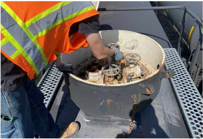
Figure A6. Inside the protective housing on the top of the tank car. Photo by NIOSH.
