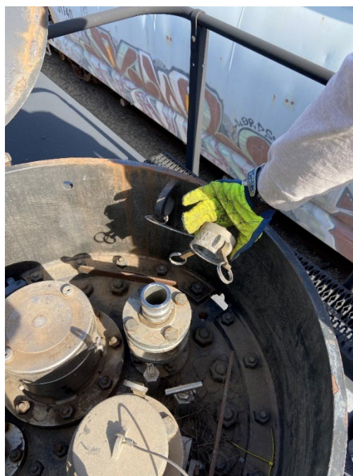
Figure B10. An open valve inside of the housing. Photo by NIOSH.
