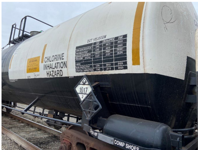
Figure B11. Chlorine tank car labeled inhalation hazard, including the inhalation pictogram on the DOT placard. Photo by NIOSH.
