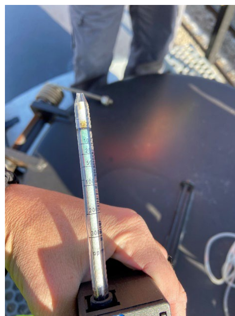
Figure B14. Colorimetric indicator tube for petroleum hydrocarbons showing ~50 ppm. Photo by NIOSH.
