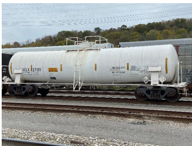
Figure A2. Cylindrical hazardous materials tank car. Photo by NIOSH.
