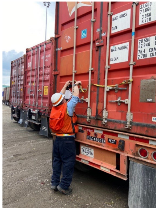
Figure A8. Inspection of an intermodal shipping container containing hazardous materials. Photo by NIOSH.
