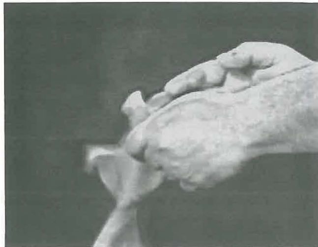
Figure 1. Dust produced by removing a latex glove containing powder.
