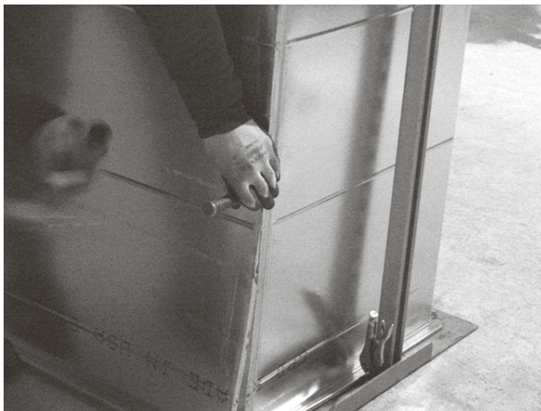
Figure 2-5.2. Tacking duct together
