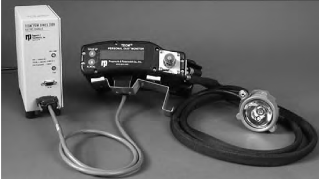
Figure 2.—Precommercial PDM connected to white docking station ( left ) used for charging and communication with a PC using an RS-232 interface.
