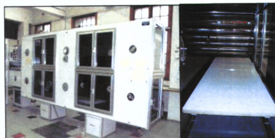
Figure 1: Pictorial view of the Polley duct with a rectangular rolling sampling table (right)
