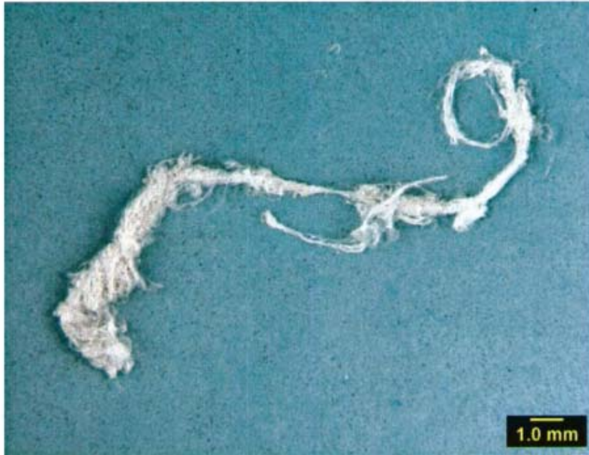
Optical Image of Chrysotile Grade 3 (textile grade).
