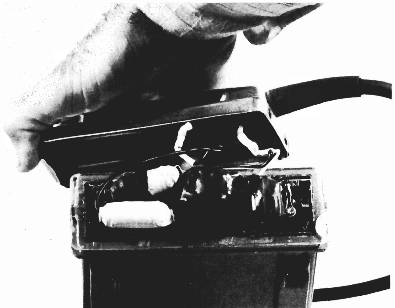
FIGURE 15. - Transmitter placed inside cap lamp battery.
