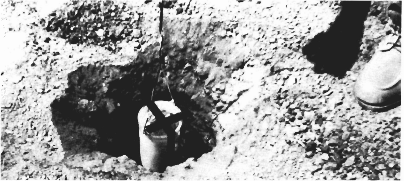
FIGURE 10. - Transmitter being lowered into test hole.
