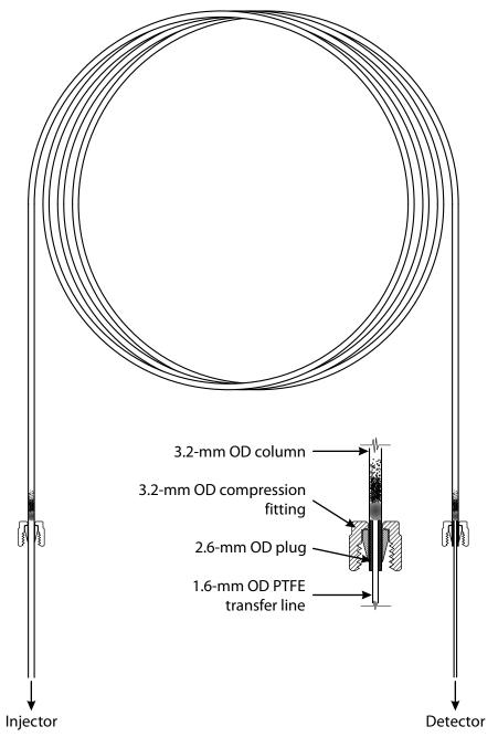
Figure 1. All-PTFE gas chromatograph system used for the determination of acetone cyanohydrin.
