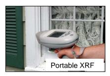
Instructor Note: Picture from Niton the manufacturer. Transporting XRF instruments across international boundaries may require additional approvals because of the cobalt source in the instrument.
