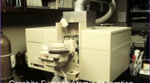
Graphite Furnace Atomic Absorption Spectrophotometry
