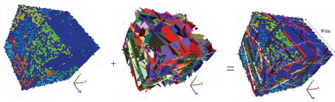
Figure 4.—A synthetic rock mass “sample” (right) is created by superimposing a stochastically defined discrete fracture network (center) onto a PFC3D particle solid (left).
