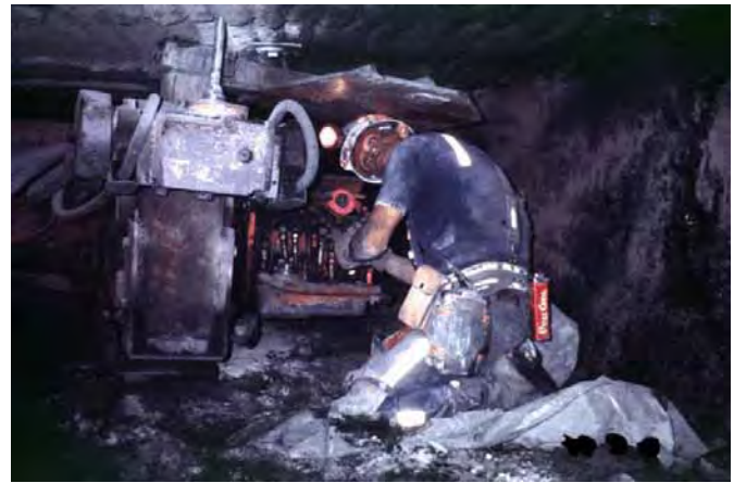
Figure 5.—A roof bolter operator's work posture in an underground coal mine.
