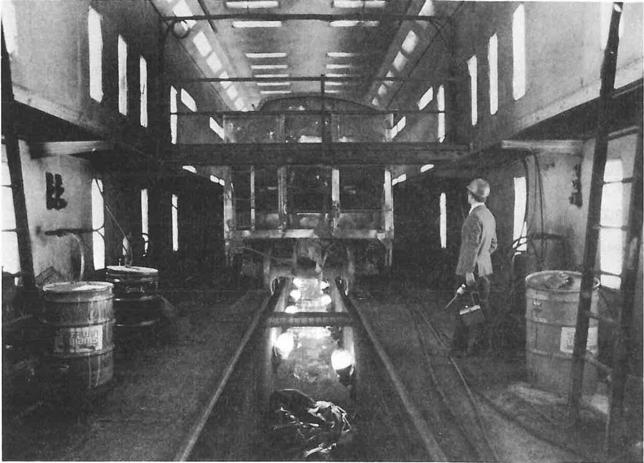
Figure 4-1. Railroad car in booth ready for painting.
