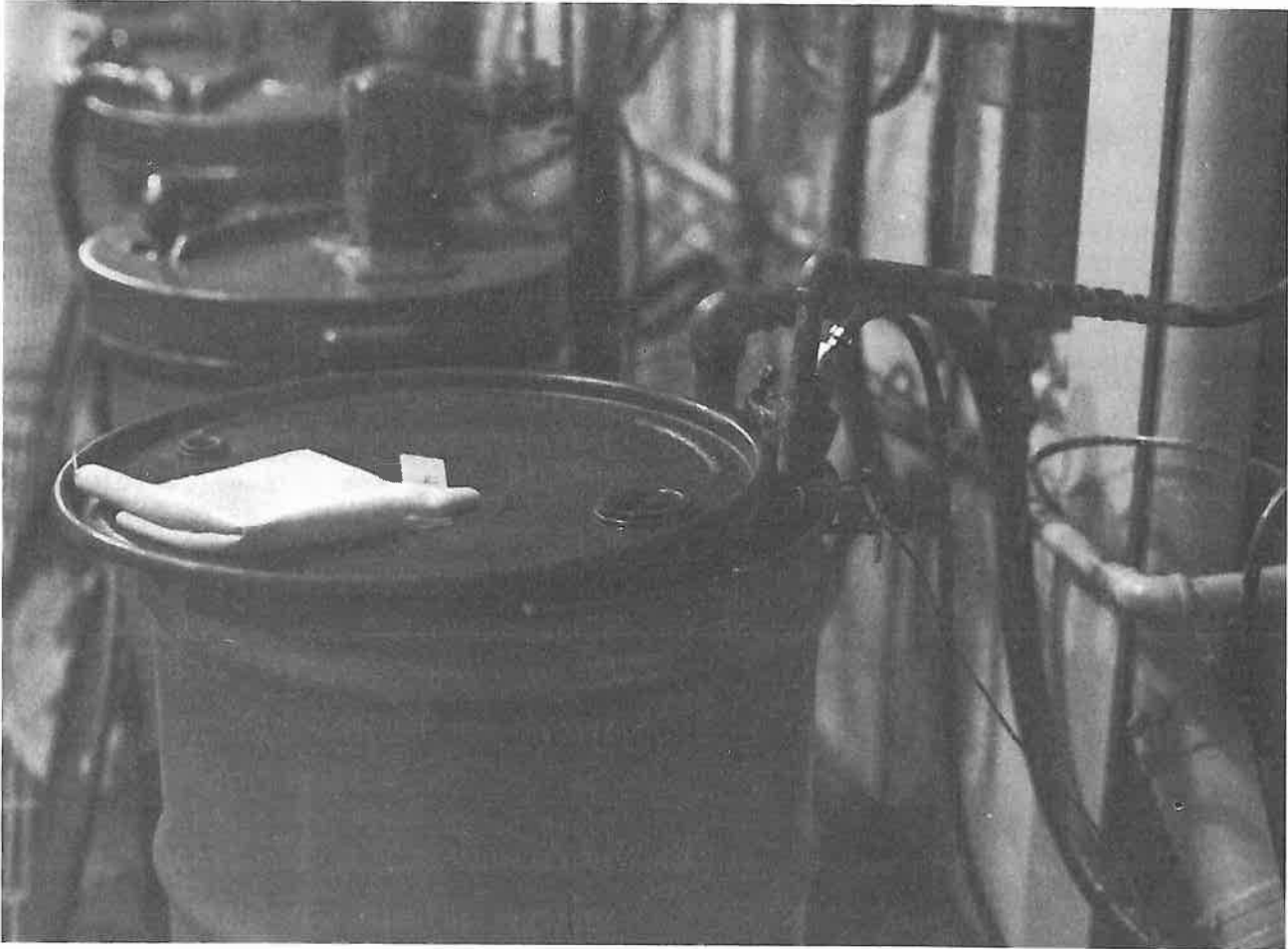
Figure 10-3. Paint mixing drum with loose fitting lid and clamp-on agitator.
