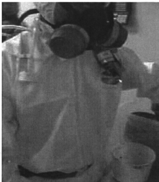
Location of personal breathing zone air sampling cassettes (Image courtesy of Mark Methner, NIOSH)
